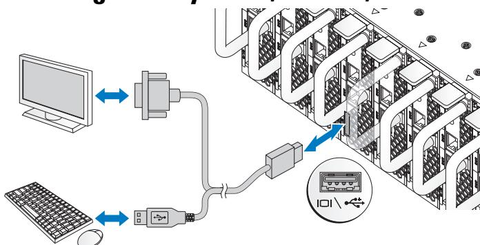
The connector on the front of your system has an icon indicating which cable to plug in. Connect a keyboard, mouse, or monitor (optional).
